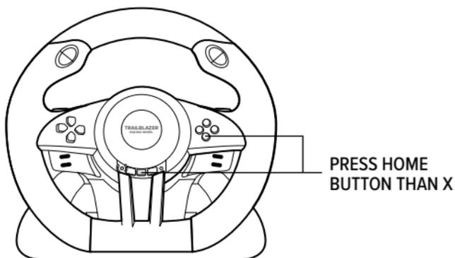
1. First connect the USB cable to the PS4\* for power supply, then use the micro-USB cable to connect the **original PS4\* gamepad** to the back USB port on the racing wheel. Now switch the console on. The LED on the racing wheel will glow red.
